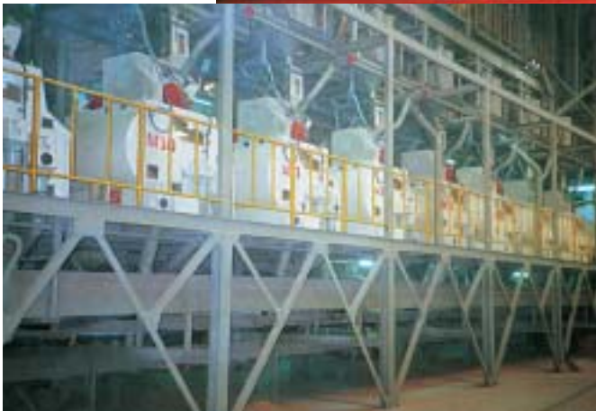
Combination of 8 Combihulls in a Rice Mill in Thailand
